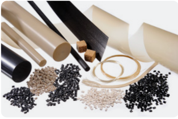
Figure 2: PEEK polymer available in a wide range of forms for use in different manufacturing processes.
