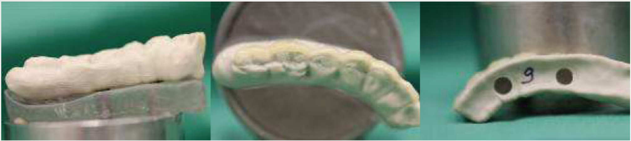
Figure 3: Restorations were fixed on an artificial jaw with simulated dental implants.
