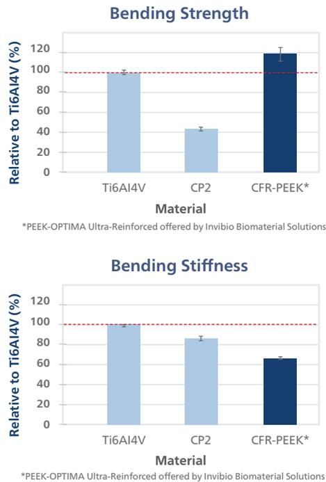
*Figure 3: Results of 4-point bend testing relative to performance of Ti6Al4V. In the test, PEEK-OPTIMA Ultra-Reinforced demonstrated greater bending strength and lower bending stiffness.*
