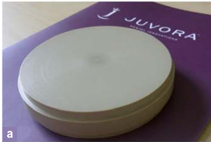
Fig. 13a and b The virtual structure was realised using CAD/CAM-assisted fabrication (PEEK, material blank: Juvora Dental Disc).
