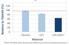
Figure 3: Results of 4-point bend testing relative to performance of Ti6Al4V. In the test, PEEK-OPTIMA Ultra-Reinforced demonstrated greater bending strength and lower bending stiffness.
